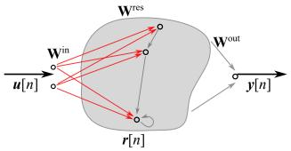
(a) K-Means-based ESN when  $K = N^{\text{res}} = 3$ .
