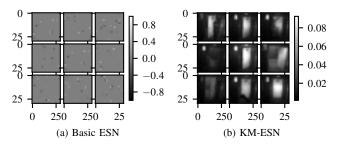
Fig. 4. Input weights for both ESN models. In case of the basic ESN (Fig. 4a), every neuron received  $\approx 10$  randomly selected input features and thus has  $\approx 890$  zero connections. The remaining values are uniformly distributed between  $\pm 1.$  In case of the KM-ESN (Fig. 4b), the weights were learned from the training dataset and represent basically mean values of various images.
