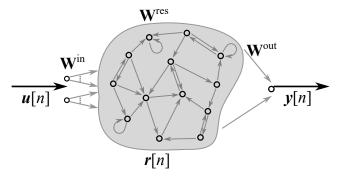
Fig. 1. Main components of a basic ESN: The input features  $\mathbf{u}[n]$  are fed into the reservoir using the fixed input weight matrix  $\mathbf{W}^{\text{in}}$ . The reservoir consists of unordered neurons, sparsely inter-connected via the fixed reservoir matrix  $\mathbf{W}^{\text{res}}$ . The output  $\mathbf{y}[n]$  is a linear combination of the reservoir states  $\mathbf{r}[n]$  based on the output weight matrix  $\mathbf{W}^{\text{out}}$ , which is trained using linear regression.
